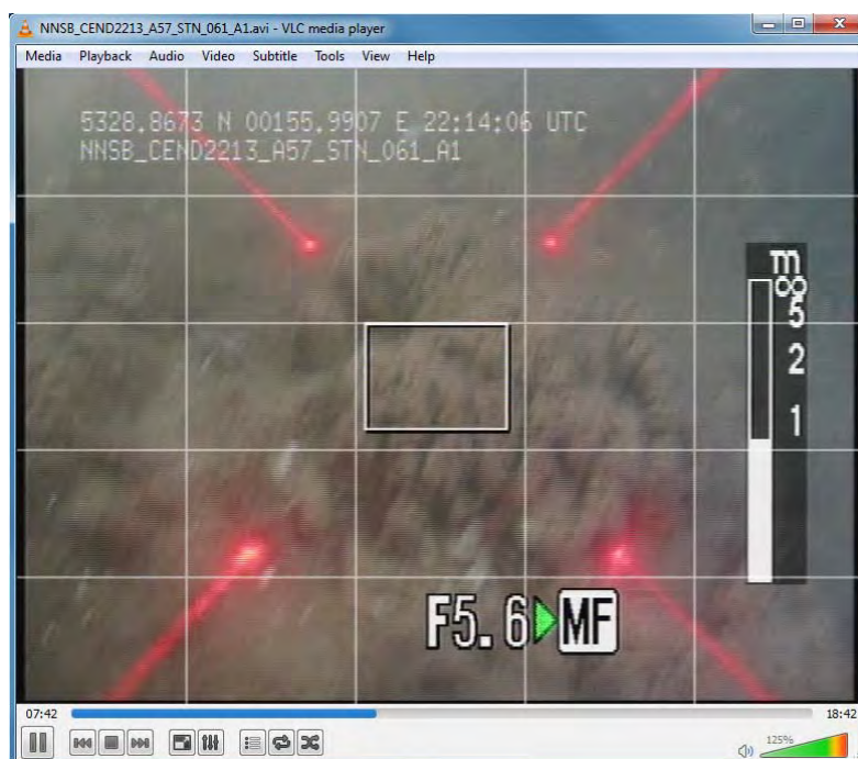
Figure A.1. Example of a transparent 5x5 grid composited over a video tow using VLC media player. Each grid cell represents 4% of the image.
